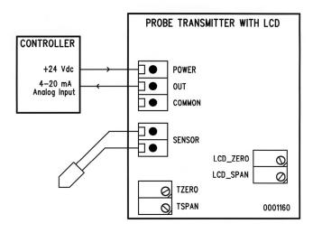
Voltage Connection With Controller 24 Vdc Power
