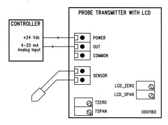
Voltage Connection With Controller 24 Vdc Power
