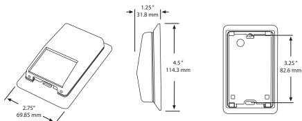
The RH100B series uses a highly accurate and reliable Thermoset Polymer based capacitance humidity sensor and state-of-the-art digital linearization and temperature compensated cicuitry in an attractive, low profile enclosure to monitor room humidity levels. An optional temperature sensor is available.
