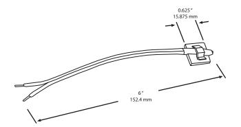
The TE200HC series incorporates a precision temperature sensor used to monitor temperatures in a variety of applications. It comes with a self-adhesive mounting clip which can be secured to almost any surface.
